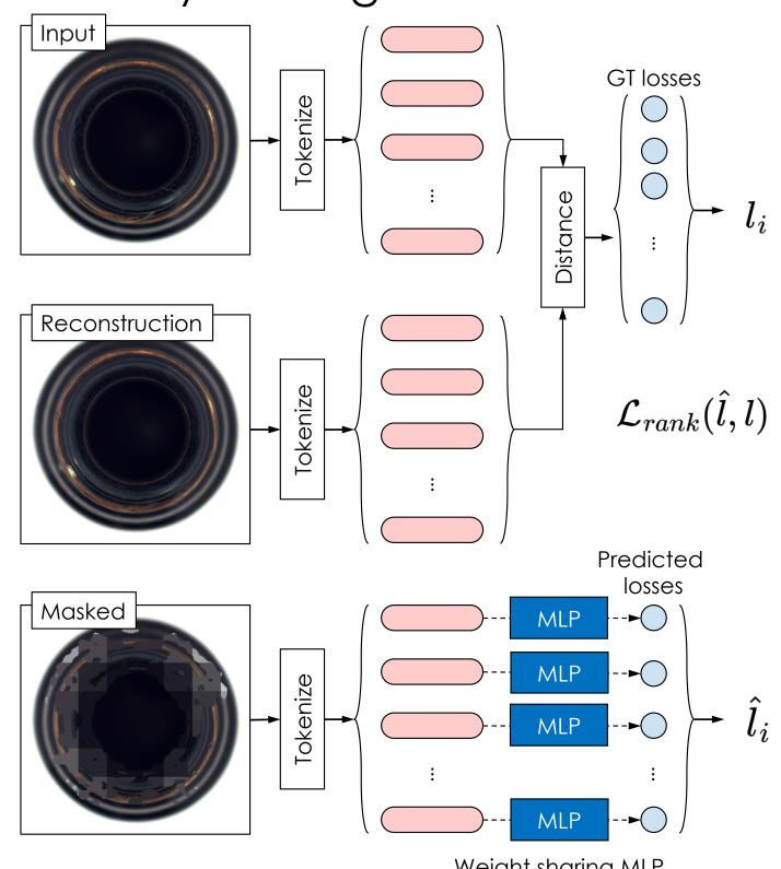
Generates a soft mask only with a simple two-layered MLP to attenuate defective representations
